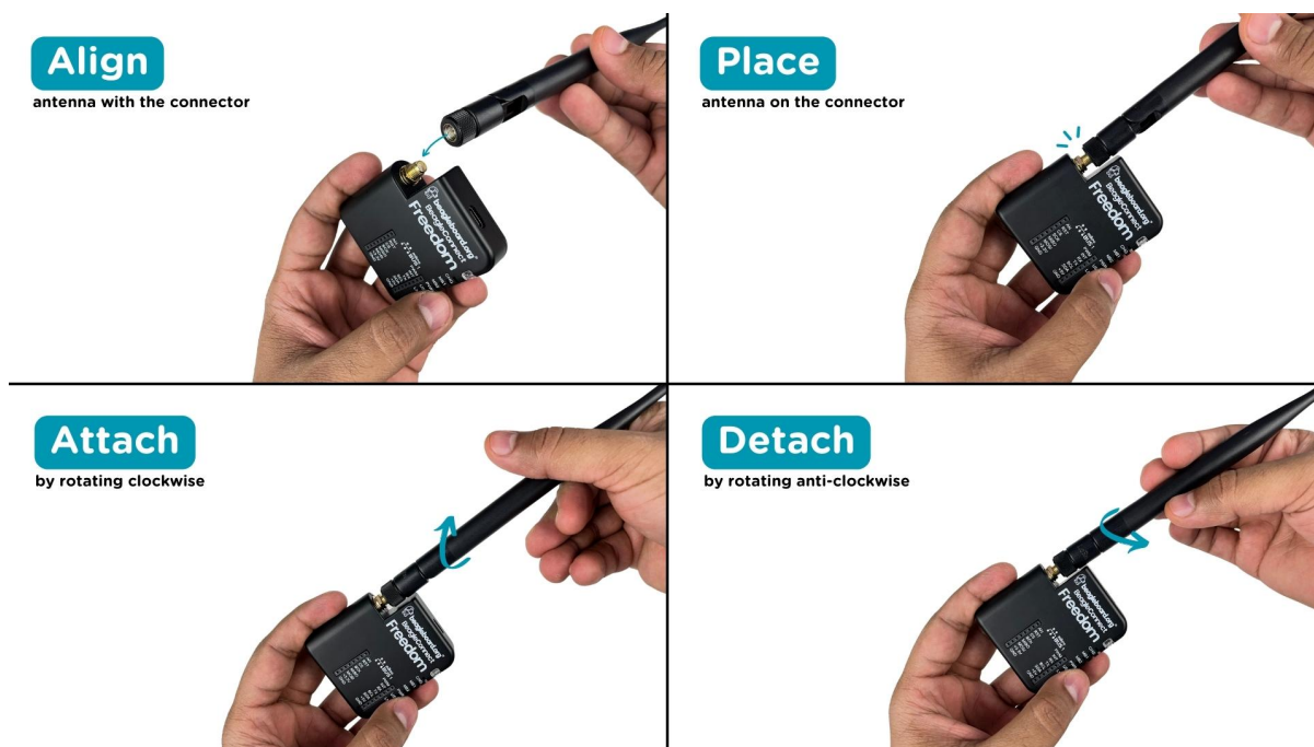
Fig. 2.2: Attaching antenna to BeagleConnect Freedom
