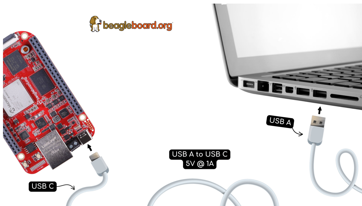
Fig. 2.2: BeagleV-Fire tethered connection
