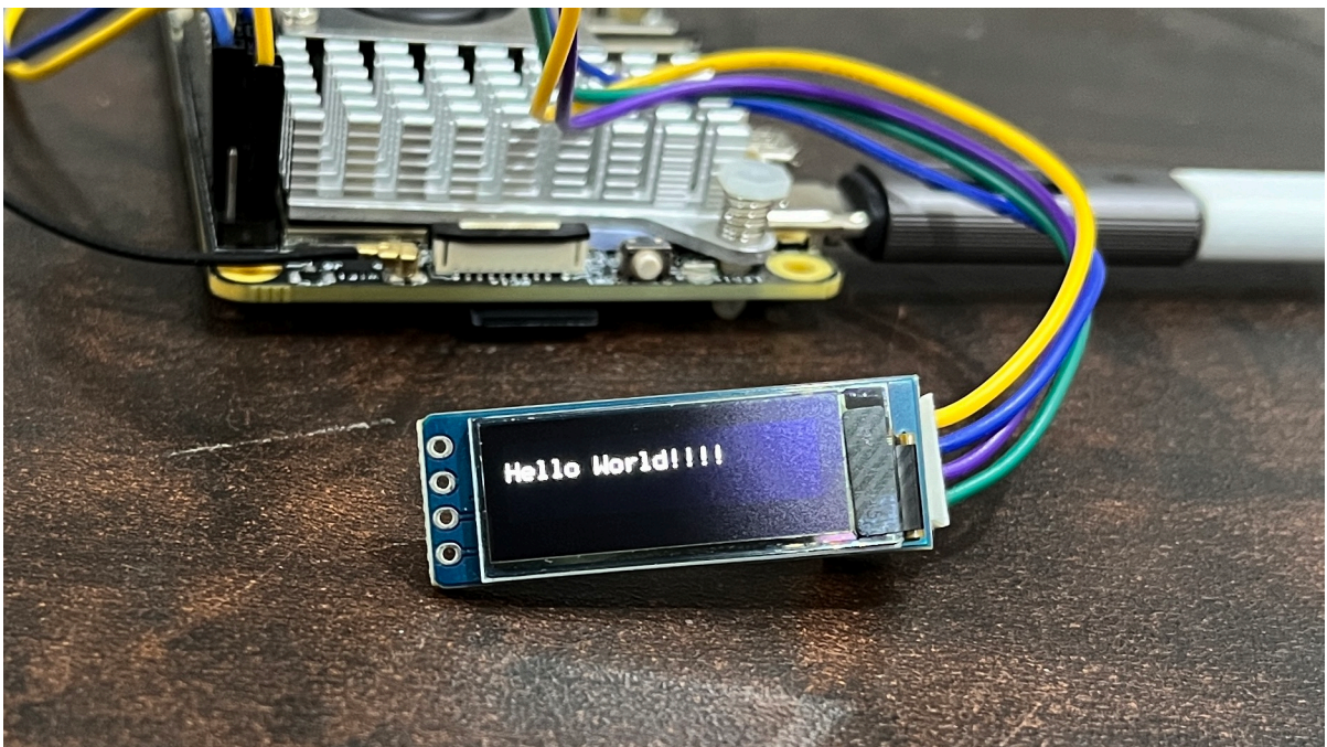
Fig. 5.22: Hello World!!!! on 128x32 OLED
